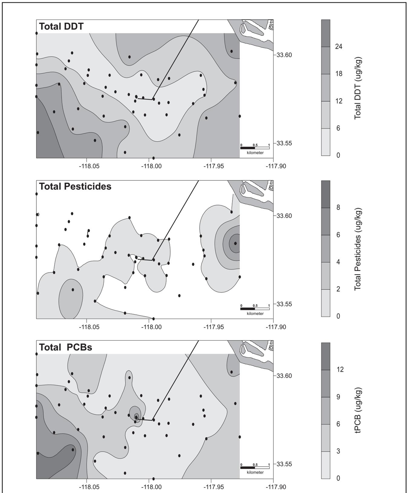
**Figure 4-5. Spatial distributions of total DDT (tDDT), total pesticides, and total PCB (tPCB) concentrations (ug/kg) during July 2009.**
