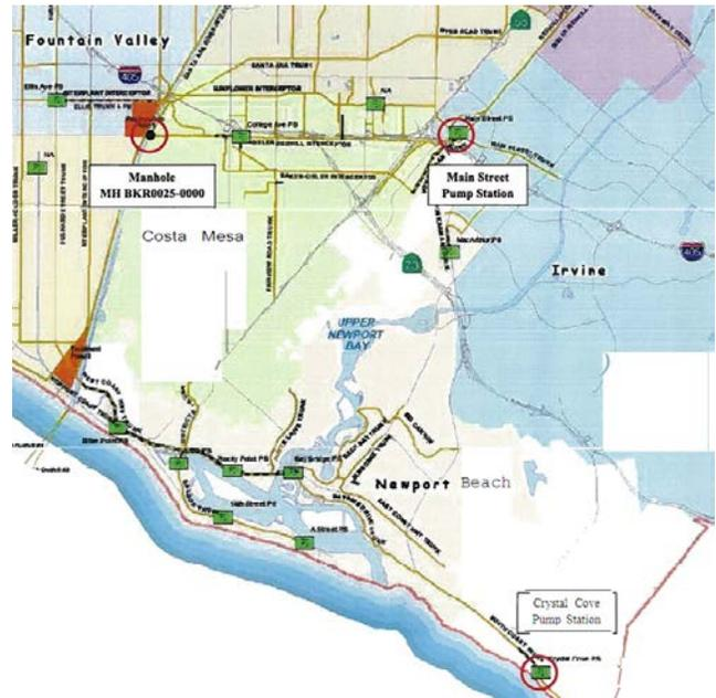
Based on the results of the data analysis, the implementation of a superoxygenation system at the Main Street pump station would be effective at controlling sulfides at the discharge of the force main and through an appreciable distance in the downstream gravity sewer. Computer modeling suggested that oxygen could not be the sole downstream odor
